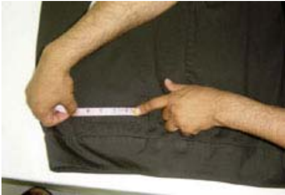
Measuring back vent height.
